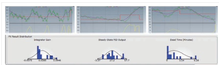
Figure 3 - Select CLPM solutions automatically capture both closed-loop set point changes and open-loop output changes, calculating models of the associated process dynamics. Aggregated modeling data offers a comprehensive view of a given control loop's behavior and it provides the basis for tuning values suitable for controlling that same range of behavior.
