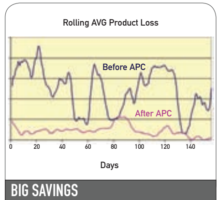
Figure 3: Among the two projects’ multiple gains, the second’s advanced process control (APC) greatly reduced product loss in the C5 refinery/isoprene unit’s distillation process.
