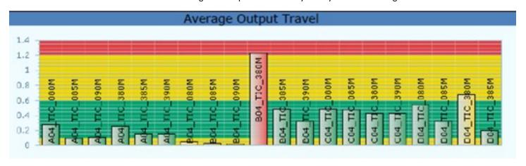
PlantESP reports include those that assess the performance of individual PID control loops or assets as well as those that compare the performance of multiple loops or assets. The image above showcases a section of one report that focuses on Output Travel. It revealed a valve that was working excessively compared to others, and it allowed engineering staff to proactively address the situation.
