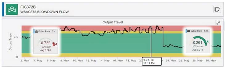
Output Travel is one of several Key Performance Indices (KPIs) used by PlantESP to assess asset health. It measures the amount of effort applied by an FCE to maintain control. The trend shows a steady increase in Output Travel with it approaching a constraint at 72.2% of its daily limit. Once addressed by engineers the KPI dropped to 26.1%, extending the valve's mean time to failure by nearly 3x.
