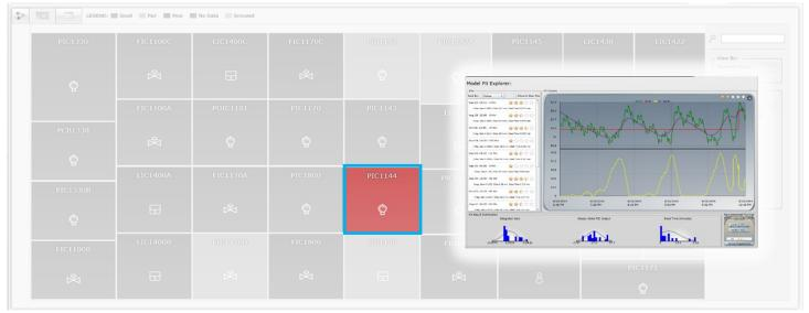
PriorityVue's color coding made it easy to single out the Medium Pressure Steam Separator loop. Performance data was examined by the customer in the context of Tuning Deviation – one of PriorityVue's many KPI filters that evaluate controller tunings. With just two clicks of the mouse the user confirmed PlantESP's assessment and examined the numerous model fits which had been calculated using the data from everyday output changes.
